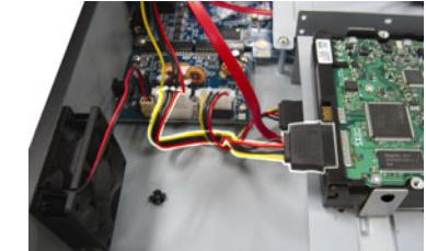
**Note:** Make sure the HDD power cable is connected to the **WHITE** jack on the DVR mainboard as shown below. The black jack is reserved for DVD writer installation.
