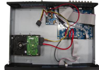
Step 4: Connect the power connector and data bus connector to the HDD.
