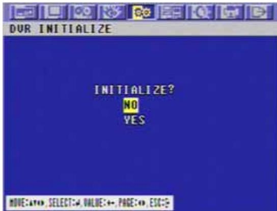
If you want to initialize, move the cursor to “YES” and then press the ENTER button. If not, move the cursor to “NO” and then press the ENTER button. Use the  $\uparrow$  ,  $\downarrow$  buttons to move the cursor. To exit this DVR INITIALIZE screen, press the ESC button.
