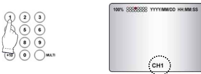
Press the desired camera number button to display on the monitor.
