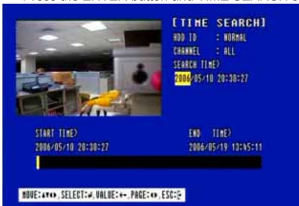
Select the desired HDD ID using the (-) or (+) button.
