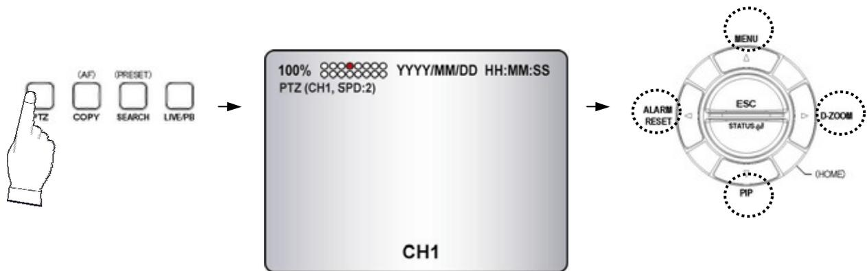
Press the “PTZ” button to control pan, tilt and zoom functions of PTZ camera.
