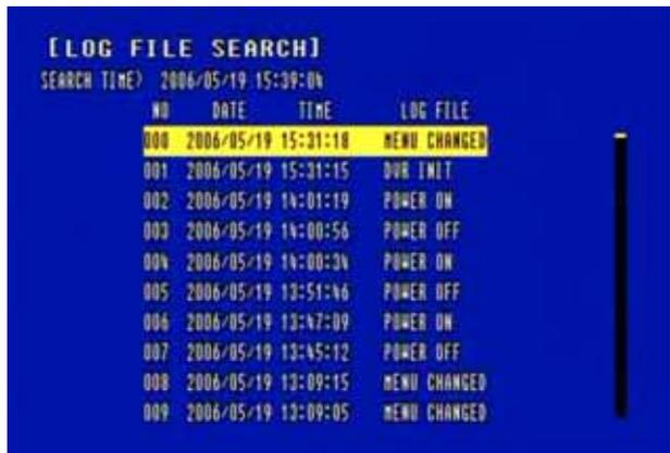
Move the cursor to the desired position of SEARCH TIME using the **↑**, **↓**, **←**, **→** buttons, and then set up the desired time using the (-), (+) buttons.
