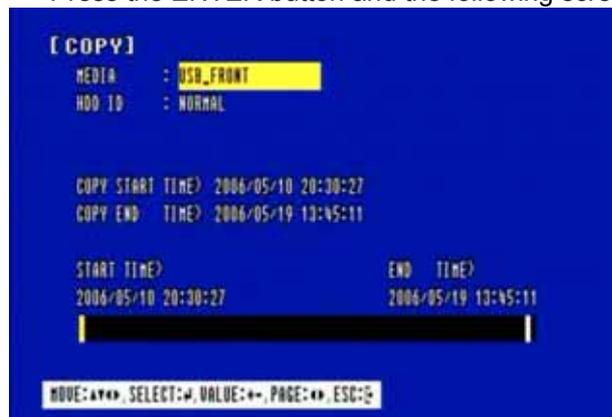
Select the desired MEDIA(select three of USB port) (-), (+) buttons or wheel scroll of mouse.
