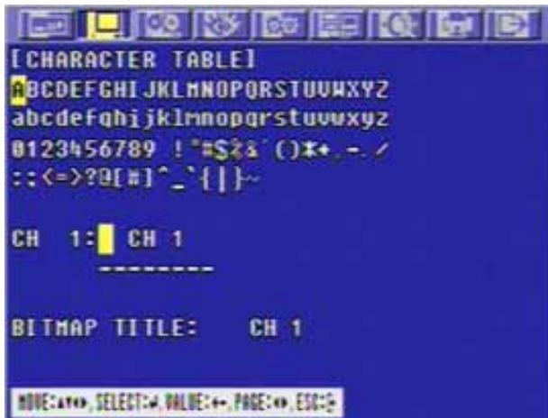
Select the character using the **↑**, **↓**, **←**, **→** buttons and then press the ENTER button. To exit this CHARACTER TABLE screen, press the ESC button.
