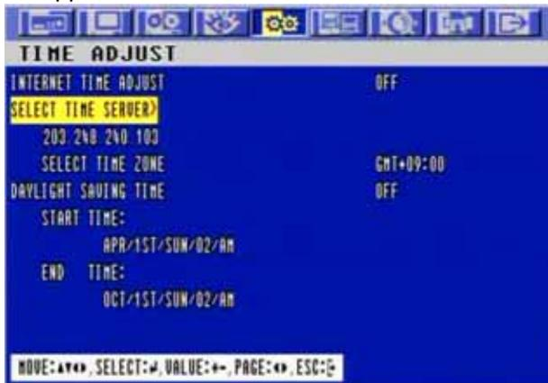
Select "ON" or "OFF" using the (-), (+) buttons or wheel scroll of mouse when the cursor is on "INTERNET TIME ADJUST". If the INTERNET TIME ADJUST is "ON", the time of DVR will be adjusted to the time offered by the internet server.
