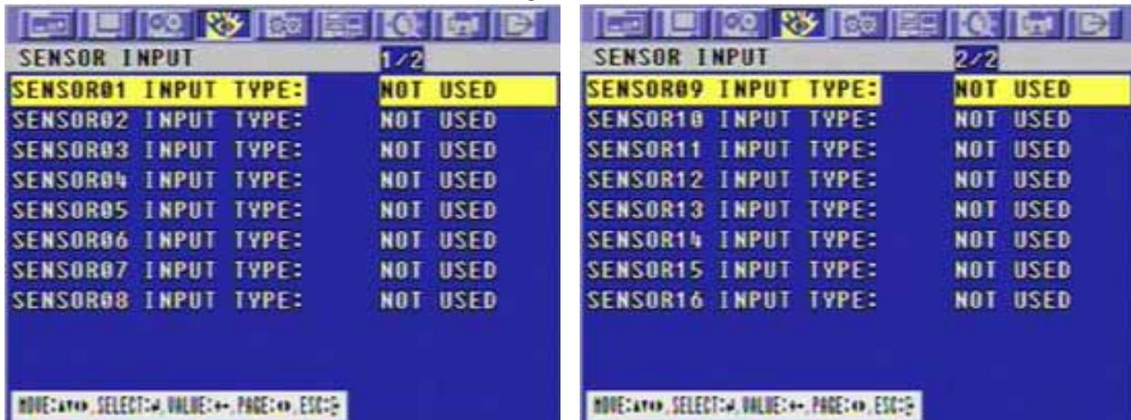
Press the ENTER button when the cursor is on the SENSOR INPUT and the following 2 pages screen appears.
