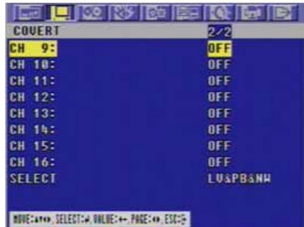
Press the ENTER button when the cursor is on the COVERT and the following 2 pages screen appears. Move the cursor and select the desired item using the  $\uparrow$  or  $\downarrow$  buttons. Use the (-), (+) buttons or wheel scroll of mouse to choose "ON" or "OFF". Use the  $\leftarrow$ ,  $\rightarrow$  buttons to see the next page.
