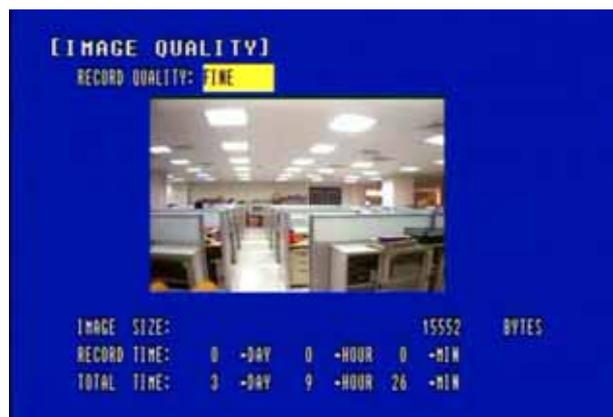
Select the desired RECORD QUALITY using the (-), (+) buttons or wheel scroll of mouse.
