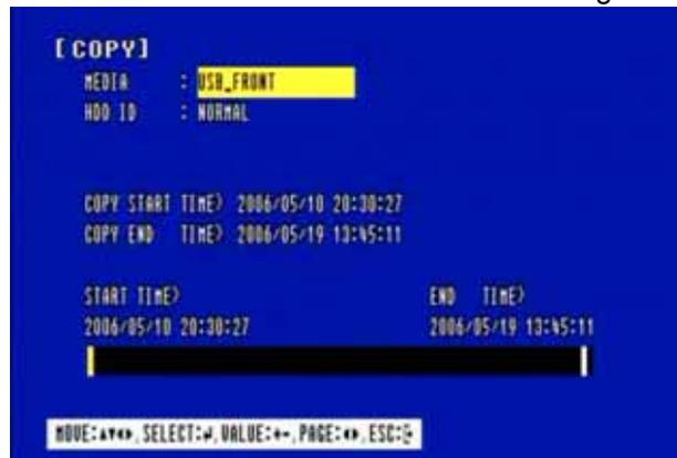
Select the desired MEDIA(USB port 3 select the correct USB position for HDD) (-), (+) buttons or wheel scroll of mouse.
