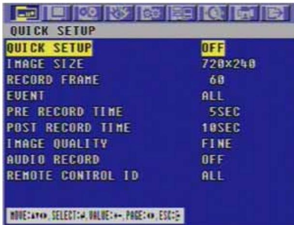
Note: If you select QUICK SETUP setting is "ON" , the DVR System will according to this Setup Page setting to record the recording data , If you select QUICK SETUP setting is "OFF", the DVR System will recording data according to the Record Setup Page setting.
