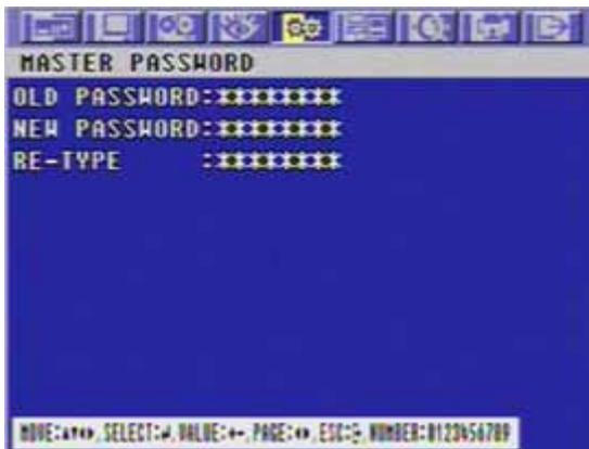
Insert the current password in the eight digits marked \*\*\*\*\* beside OLD PASSWORD using the CAMERA/ NUMBER INPUT buttons.
