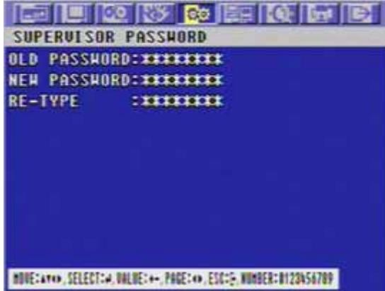
Insert the current password in the eight digits marked \*\*\*\*\* beside OLD PASSWORD using the CAMERA/ NUMBER INPUT buttons.
