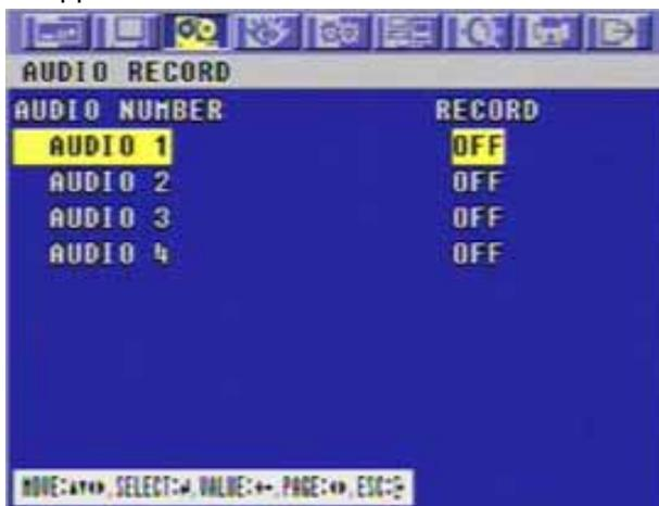
Select the recording channel for each audio channel using the (-), (+) buttons or wheel scroll of mouse.
