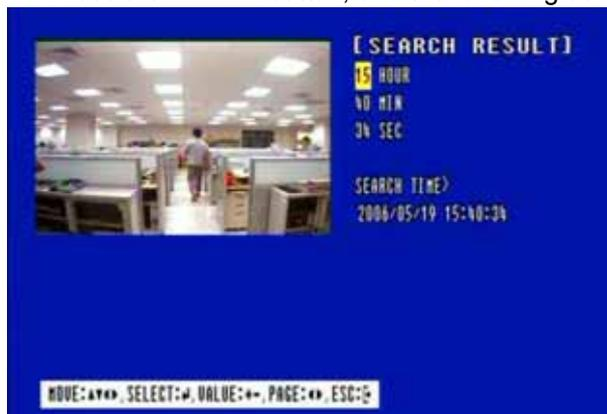
Move the cursor to the desired position of during HOUR, MIN and SEC using the **↑**, **↓**, **←**, **→** buttons, and select the desired time using the (-), (+) buttons.
