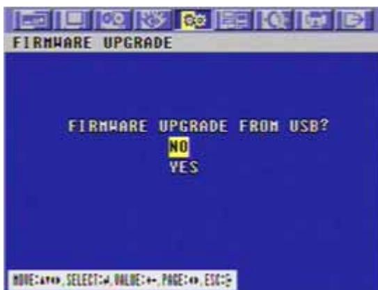
If you want to update firmware using the USB\_FRONT port, move the cursor to “YES” and then press the ENTER button. If not, move the cursor to “NO” and then press the ENTER button. Use the  $\uparrow$  ,  $\downarrow$  buttons to move the cursor. To exit this FIRMWARE UPGRADE screen, press the ESC button.
