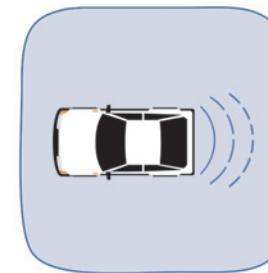
When in reverse, the 4 rear sensors installed in the back bumper send ultrasonic sound waves that bounce off objects. A display panel mounted inside the vehicle provides both visual and audible warnings to the driver regarding the distance of those objects.
